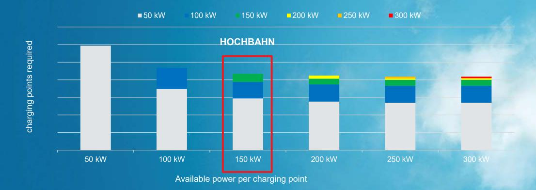
A charging power of 150 kW is sufficient for charging buses on time and the required amount of flexibility.
