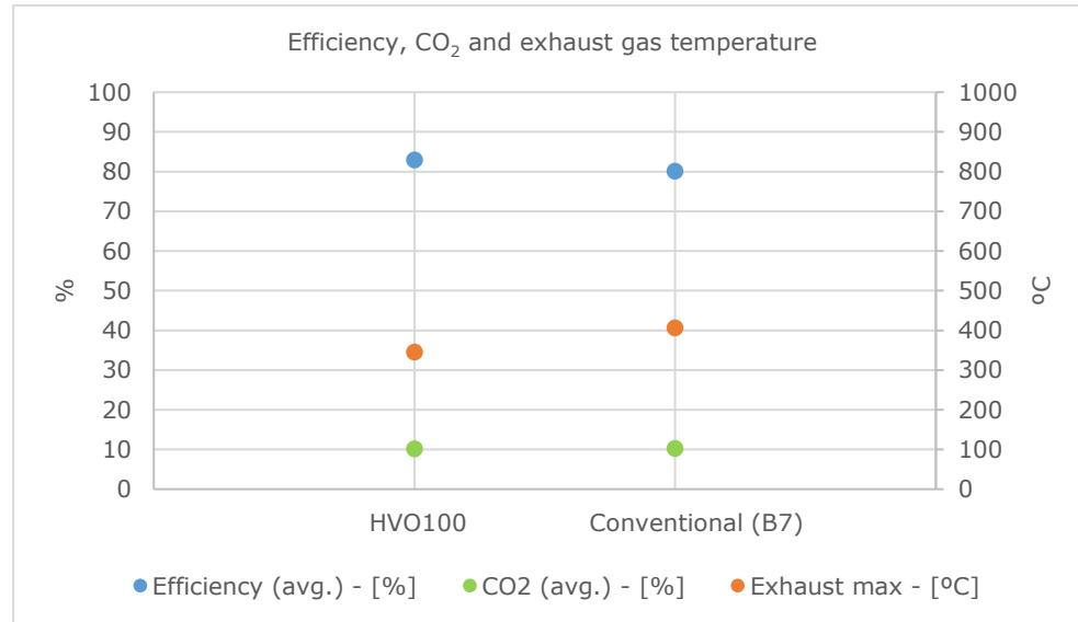
It appears that HVO100 has a slightly higher average combustion efficiency compared to conventional diesel (B7). The average CO<sub>2</sub> is almost the same for the two fuels, so the difference in combustion efficiency all comes from the lower exhaust gas temperature.
