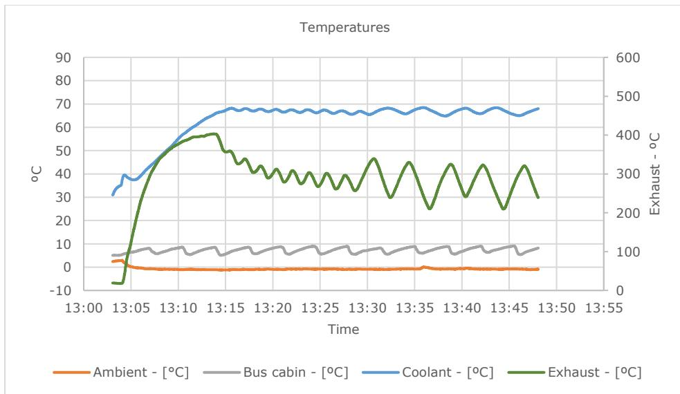
Since the start phase gives the highest emissions of CO, particles and soot, heater two is disadvantaged in comparison to heater one - because it is too efficient.
