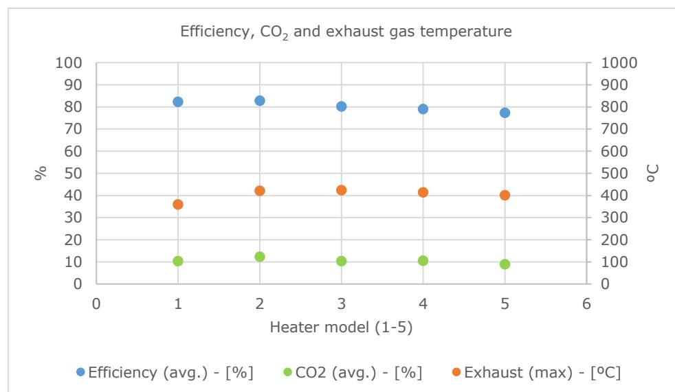
Overall, the best performance regarding combustion efficiency is delivered by model 1. It has the lowest exhaust gas temperature in combination with a CO<sub>2</sub> level almost in the middle of the recommended range, at 10,4% vol. Have in mind that this could cover a variation from too high to too low CO<sub>2</sub>.
