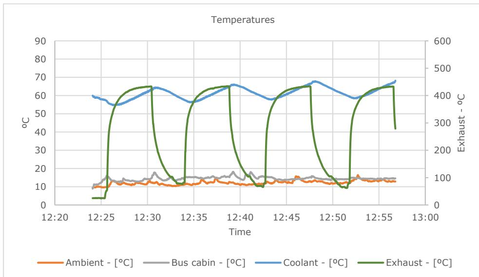
This gives very similar cycles and comparable results, and emissions and exhaust gas temperature are stable at the end of each on-period.
