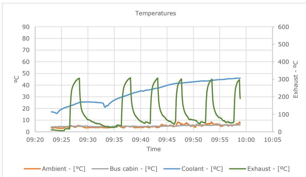
The short cycles mean that the exhaust gas temperature is not completely stable in the end of each on-phase. This must be considered when evaluating whether the exhaust gas temperature – and the combustion efficiency – is ok.
