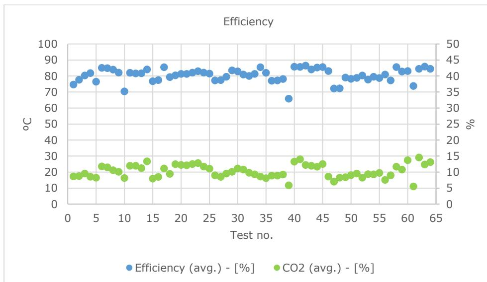
There is some correlation between exhaust gas temperature and CO<sub>2</sub>. The higher CO<sub>2</sub>, the higher combustion efficiency, but due to the combustion quality and emission of combustible gasses as CO, HC and particles, the CO<sub>2</sub> should not be higher than 11% as mentioned in
