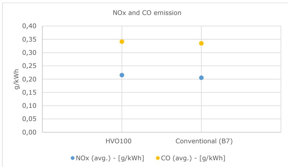
CO and NO<sub>x</sub> are almost identical for the two fuels. No significant difference is observed.
