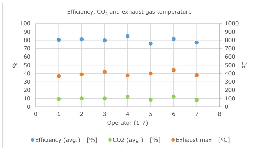
The max exhaust gas temperature varies from 368°C to 441°C from the lowest to the highest level.
