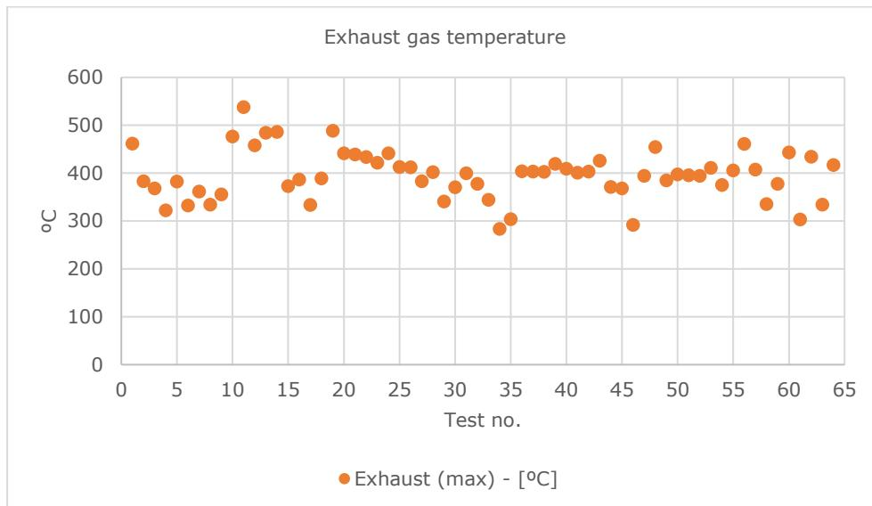
The exhaust temperature is generally very high, which indicates that most of the heaters need cleaning. Experience suggests that exhaust gas temperature should be below 350°C on a well serviced, clean and efficient heater.
