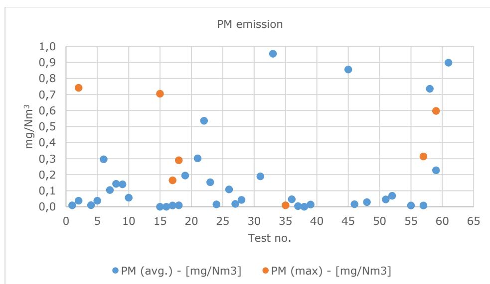
The avg. values are low in most of the tests, but some are very high. In these tests, a lot of smoke was observed, especially at the ignition phase.
