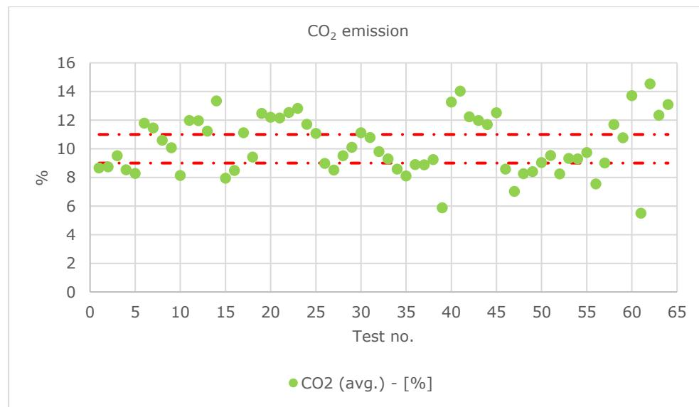
Experience suggests that heaters of this type have the best combustion when CO<sub>2</sub> is between 9 and 11%<sub>vol</sub>. As the figure shows, not many of the heaters fulfil this recommendation. 17 heaters are between 9 and 11%<sub>vol</sub>, and 47 are outside the range.
