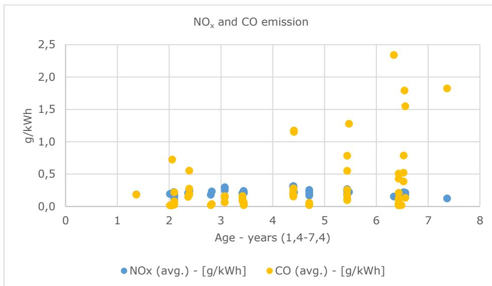
The  $NO_x$  emission is close to constant through all the heaters, independent on the heater's age.
