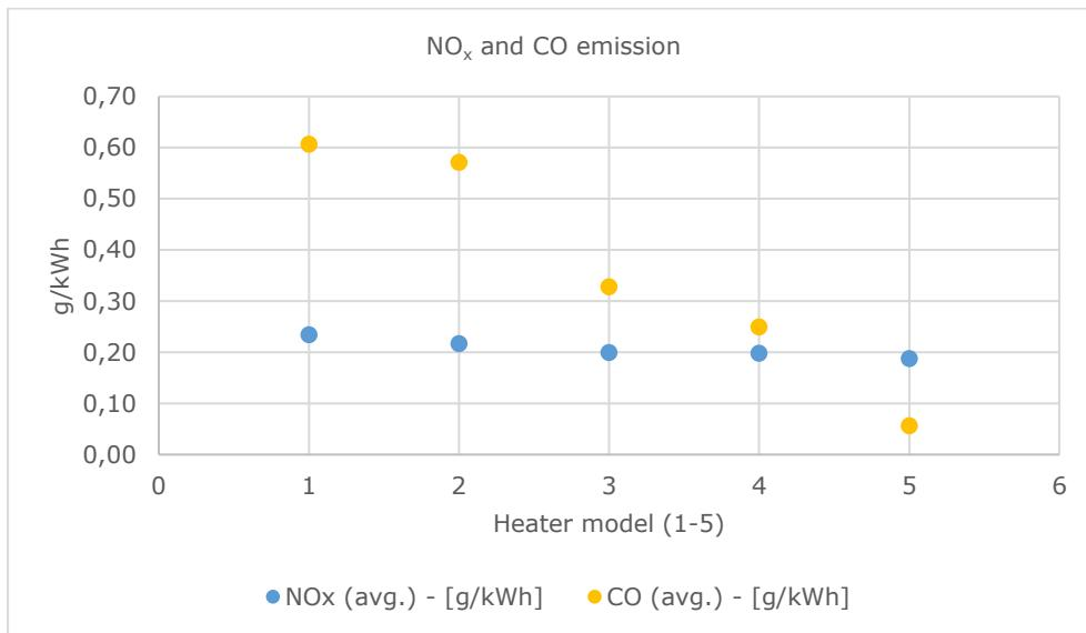
The NO<sub>x</sub> emission is roughly constant through all the heaters, independent of the heater model.
