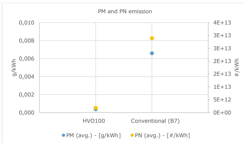
Regarding the particle emission, there is a very significant difference. As mentioned above, the heaters have been set and serviced app. to same level, so this is most likely 100% fuel depending<sup>6</sup>.
