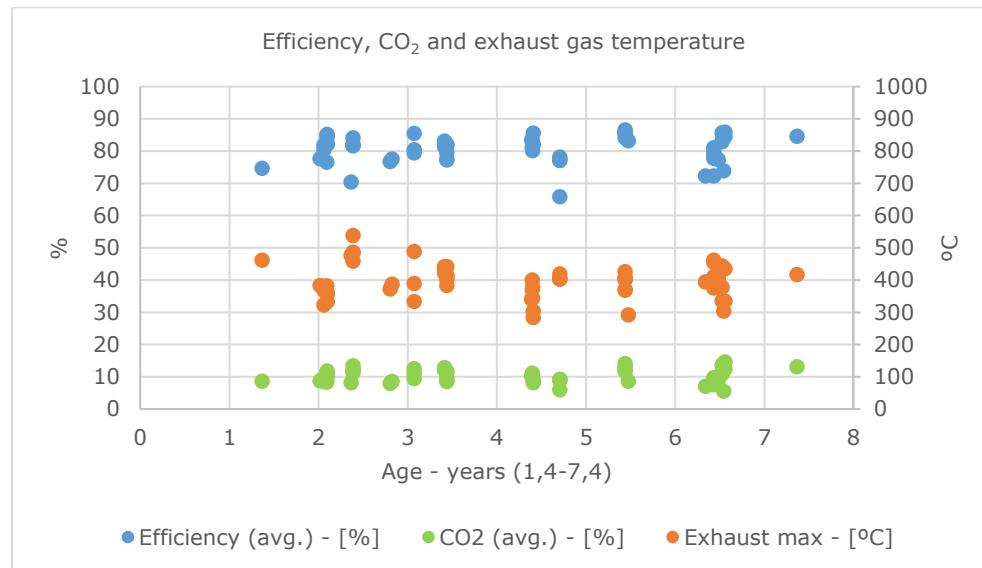
No correlation between age and exhaust gas temperature or combustion efficiency is shown. The average values are almost constant for both parameters throughout the 7-8 years range.
